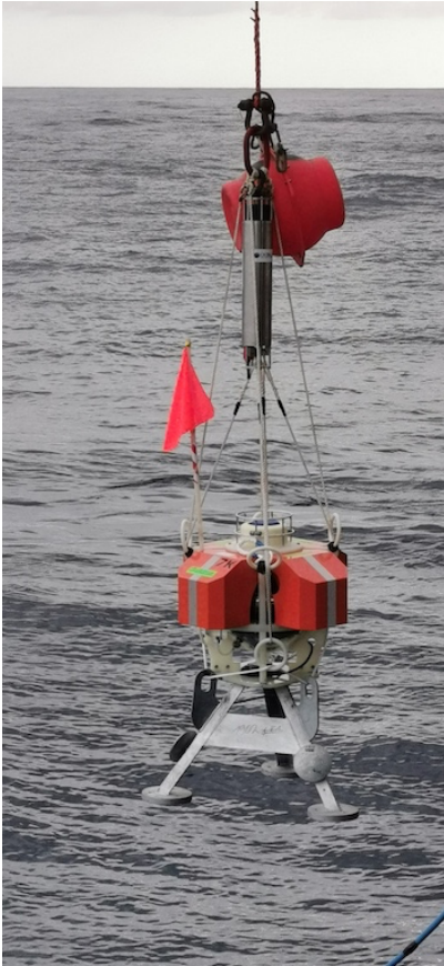
Figure 3: Photo of the drift-free pressure sensor during installation on the deep-sea wire. Photo: A. Dannowski.
