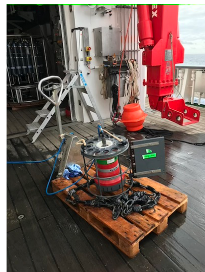
Figure 4: Photo of acoustic modem for acoustically connecting to the pressure sensors. Photo: D. Lange
