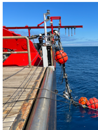
Figure 1: Retrieving the air pulsers and floats on the starboard side. Photo: B. Bauer.
