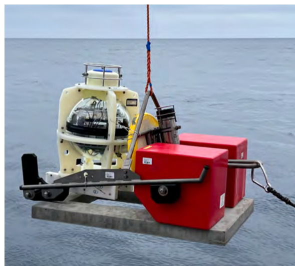
Figure 4: Floating test of the drift-free pressure sensor on a modified OBS instrument carrier. Photo: T. Bartels.
