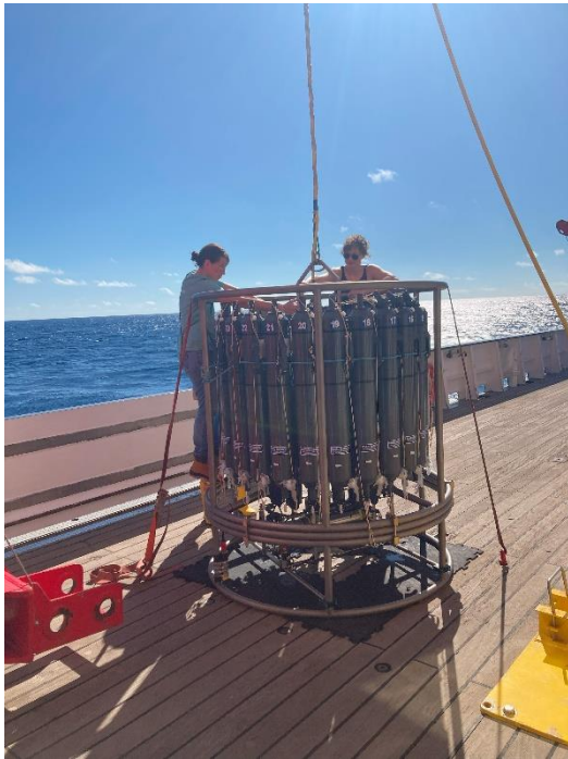
Fig. 2: Setting up trace metal clean CTD during day-light hours. Photo Lea Blum.
