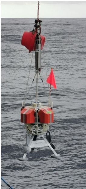
Fig. 11.6. GEOMAR Pressure sensor mounted upon an OBS frame upon deployment.
