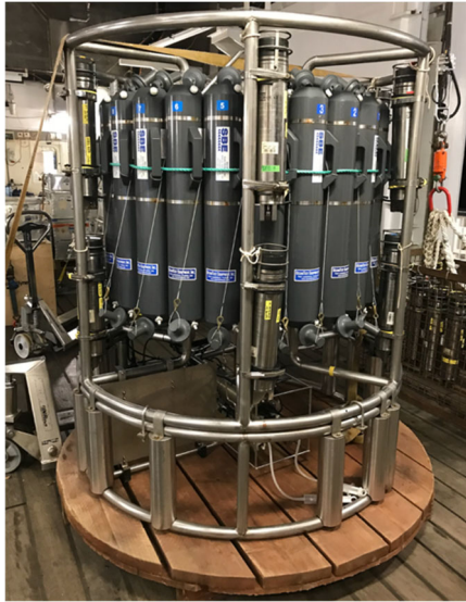
Figure 11.7 Releaser mounted on the CTD rosette for a releaser test.
