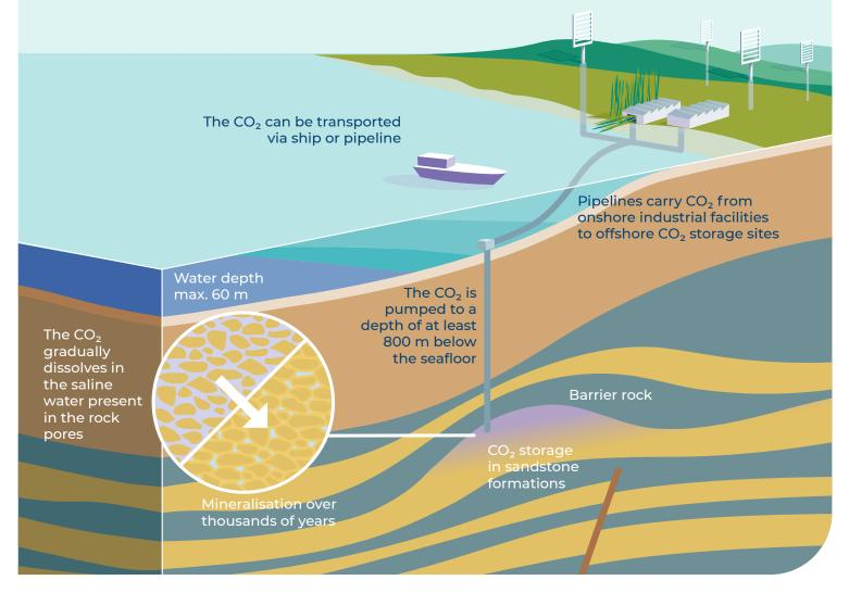
For storage in the ocean's subsurface, liquid carbon dioxide is transported by pipeline or by ship to the relevant ocean site and injected through one or more boreholes into deep porous sandstone formations. Graphic: Rita Erven, CDRmare/GEOMAR
