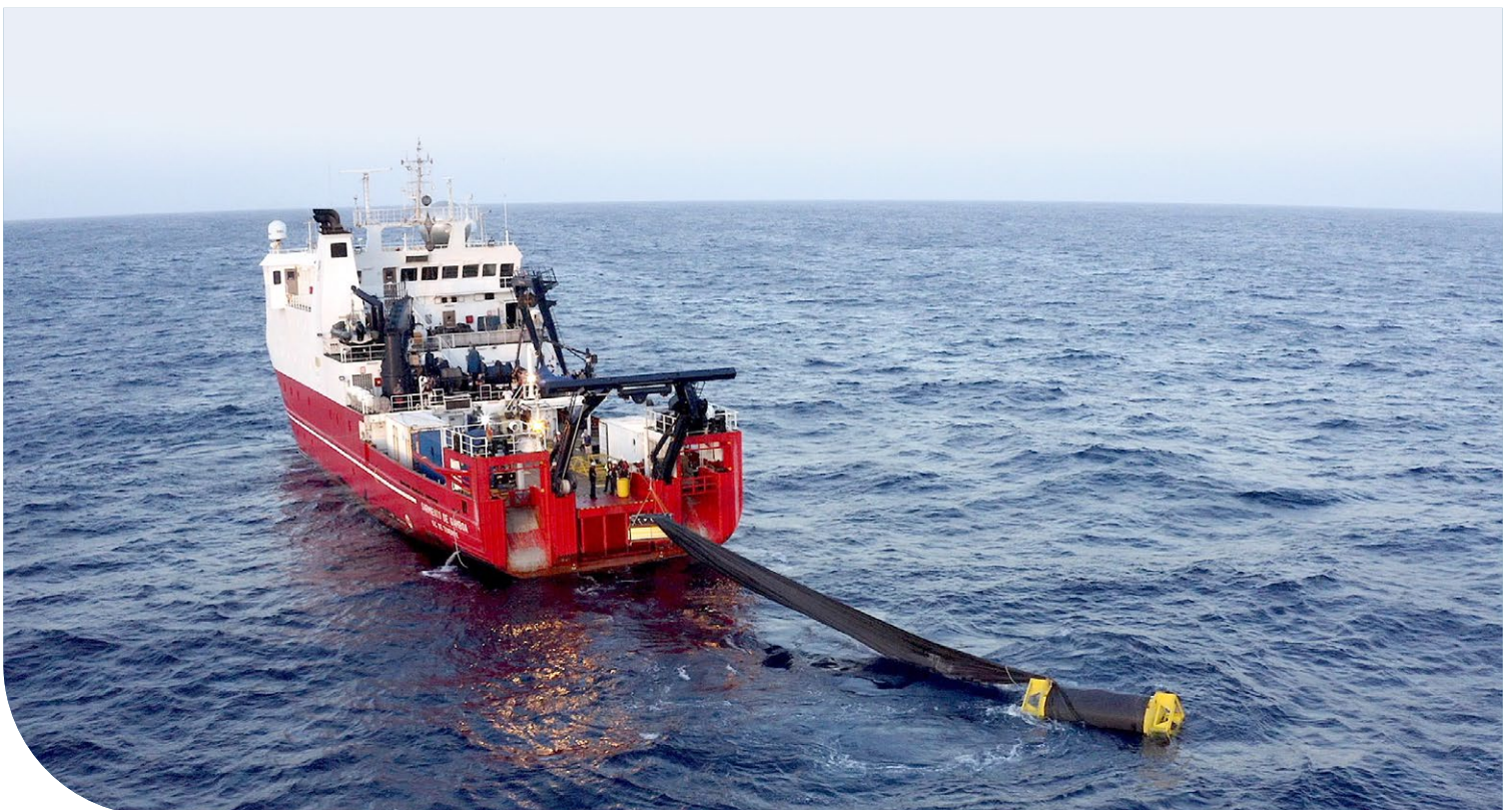
A Spanish research vessel deploys the wave pump of the research mission CDRmare for testing purposes in November 2022. Photo: D. Gutierrez
