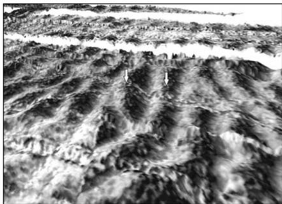
Figure 4. Three-dimensional view (toward NNW) of the backscatter map draped over bathymetry between the high-backscatter areas B and C (see Figure 3). The elevated backscatter related to the dunes typically occurs at their eastern side. The distance between the two arrows is 105 m (wavelength); the wave amplitude is 1.2 m. The image only shows the backscatter map draped over the bathymetry; no illumination is applied.
