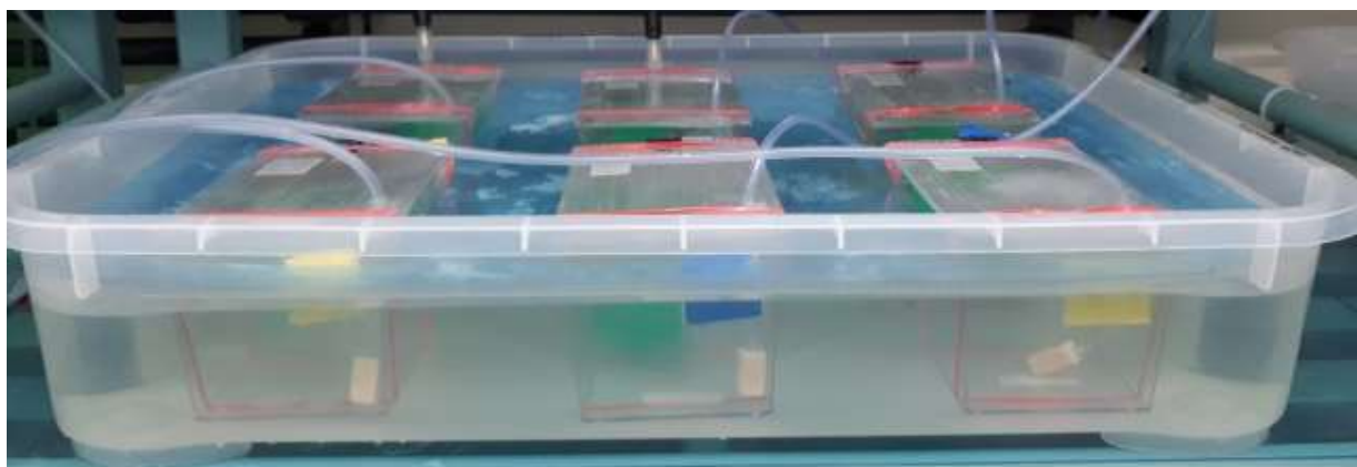
Figure 1. Experimental set up showing six experimental units in a water bath. Individual fastened plastic covers, artificial habitat, and aeration input can be observed. (Image by ©Louisa Langrehr)
