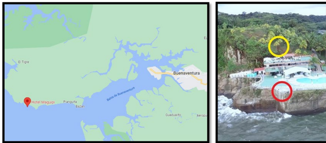
Figure 6. Agreed site for Buenaventura tide gauge installation at Hotel Maguipi. The right panel shows the planned location of tide gauge sensors (red circle) and the supplementary electronics (yellow circle)
