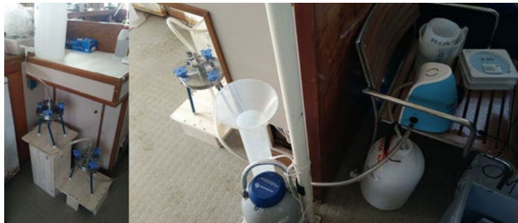
Figure 1. Pump placement in the wet lab on board
