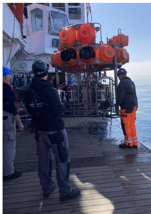
Fig. 5.4 BIGO lander system after recovery.
