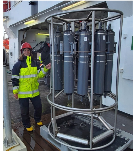
Fig. 5.2 Multi-water sampler MWS 622 before first deployment (June 5 th ).
