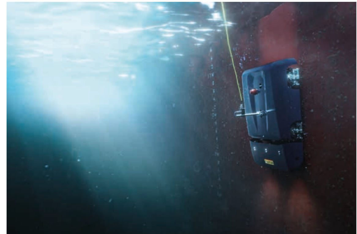
4.28 > Cleaning robots such as the HullSkater , developed in Scandinavia, will remove fouling and grime from ships' hulls with little effort in the future. Its use will eliminate the need for divers.
