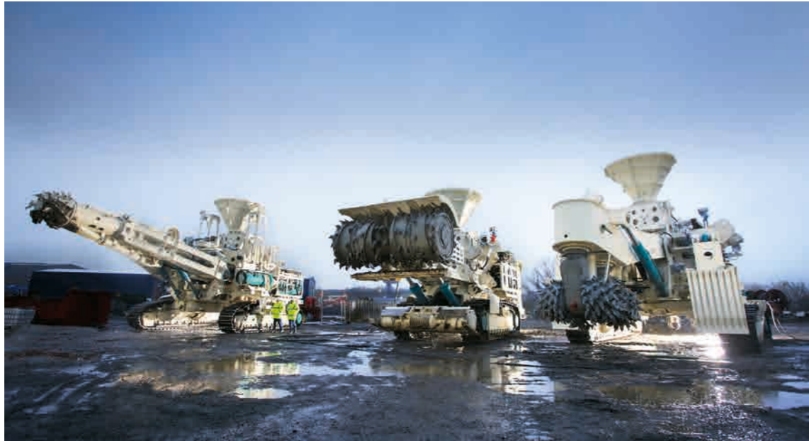
5.12 > The now bankrupt Canadian company Nautilus Minerals developed three remote-controlled underwater vehicles for mining a massive sulphide deposit in the Bismarck Sea off Papua New Guinea: a shaper (auxiliary cutter, right), a bulk cutter (centre) and a collector (left).
