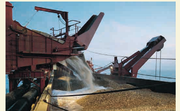
5.16 > Off the Dutch island of Ameland a suction dredger extracts sand from the bottom of the North Sea to be used in widening the island's beach.
