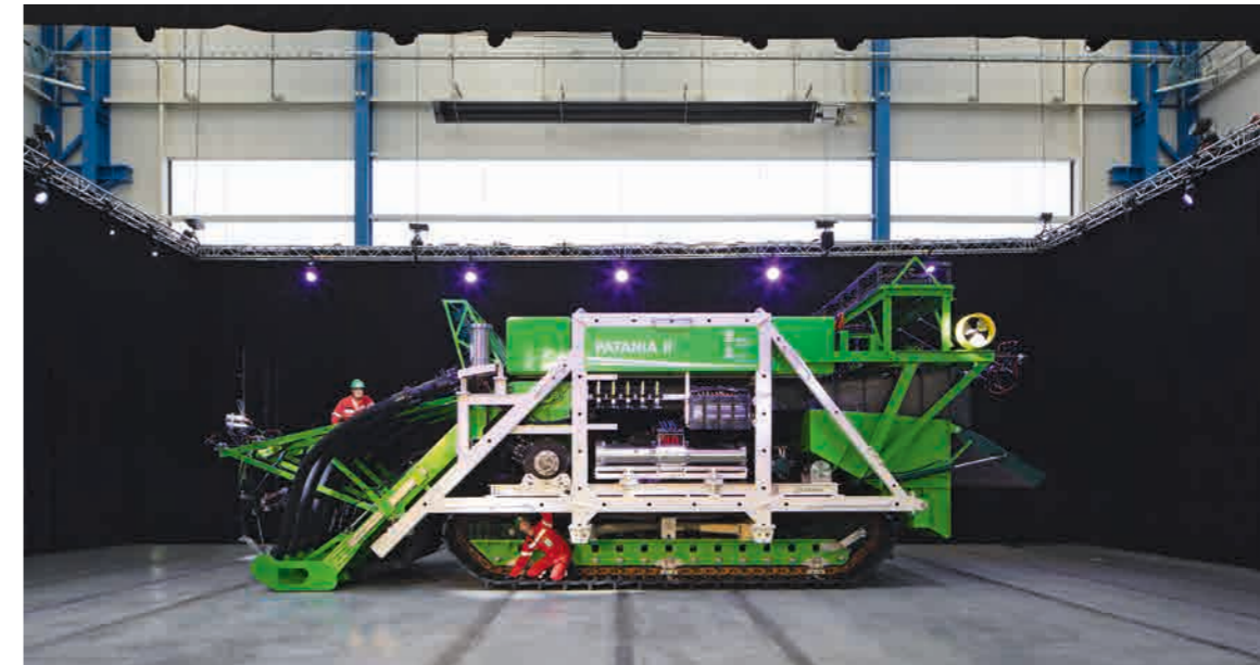
5.11 > Patania II, a caterpillar-like collector of manganese nodules made by the Belgian company DEME-GSR, is twelve metres long, 4.5 metres high, four metres wide and weighs 25 tonnes. The prototype was tested successfully in the spring of 2021 in the Clarion-Clipperton Zone at a water depth of 4500 metres.
