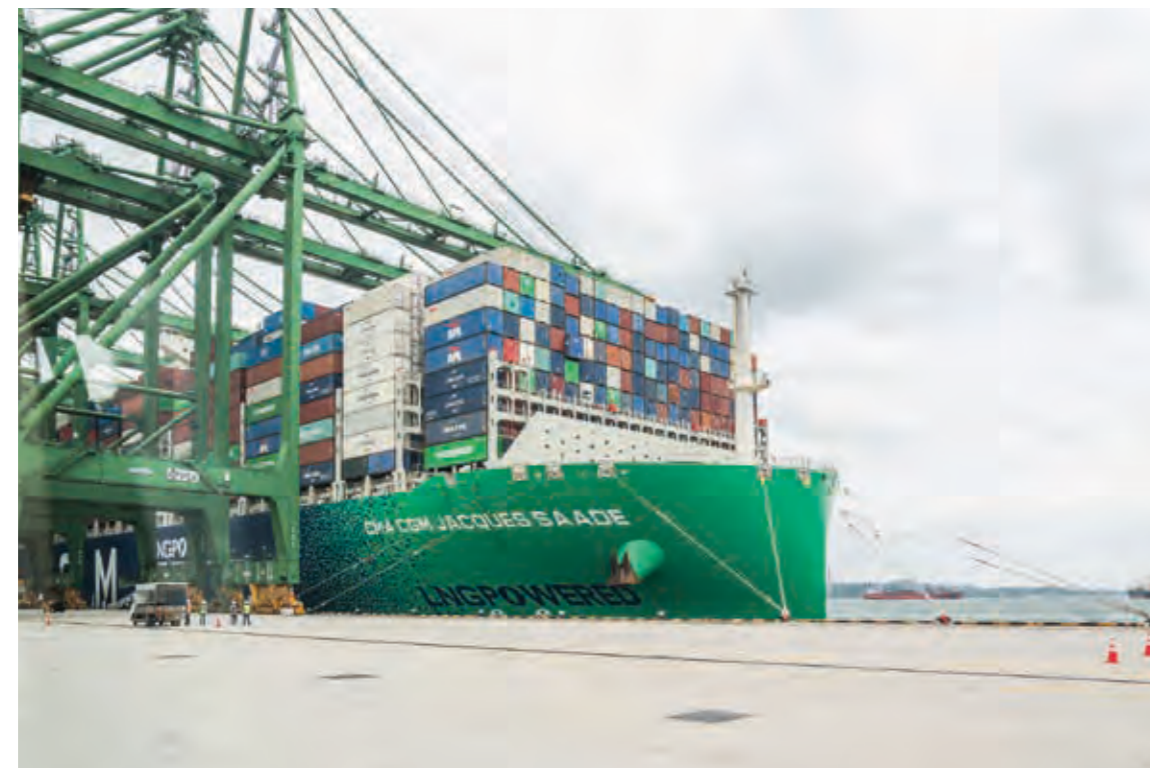
4.15 > No more black clouds of soot: The container ship Jacques Saadé , operated by the French shipping company CMA CGM, is powered by liquified gas and is presently the largest freighter with this kind of alternative propulsion system.
