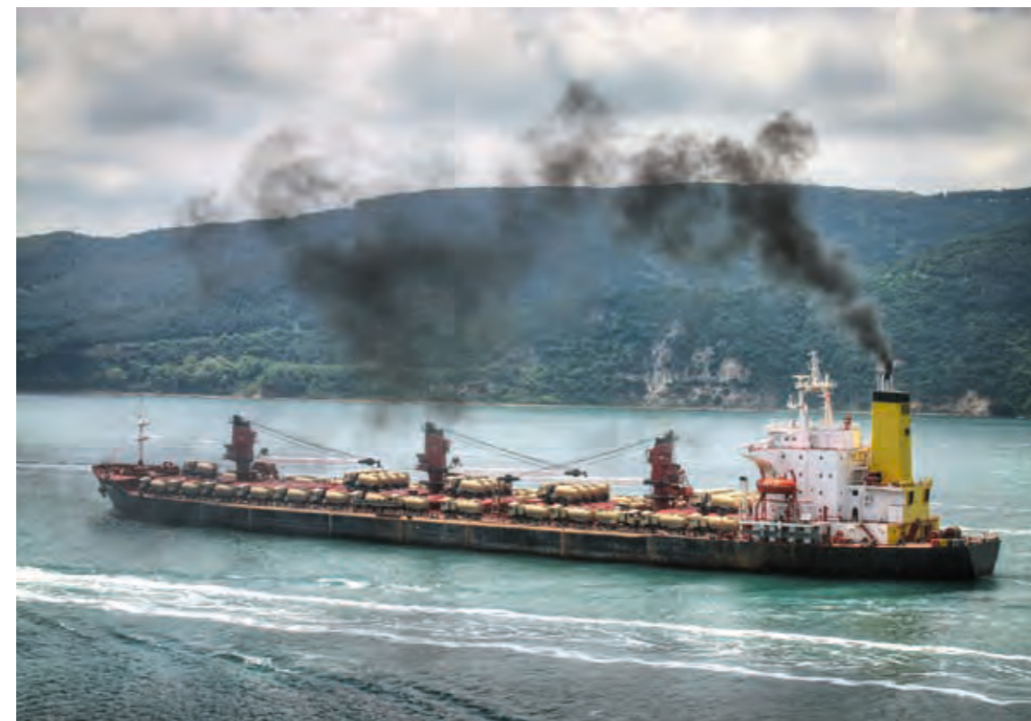
4.9 > Soot, sulphur oxides, particulate matter: Ships have been poisoning the air for decades. The seagoing vessels using heavy fuel oil as a fuel were especially problematic. Since January 2020, however, a new regulation is in effect that requires fuels to be lower in sulphur.
