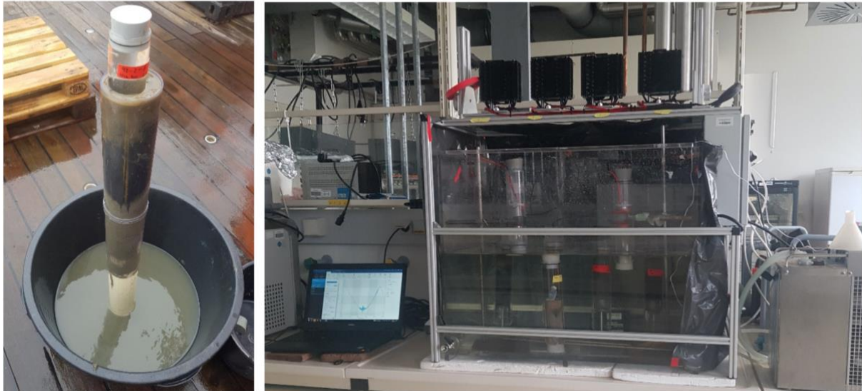
Fig. 5.3.2.1 (left panel) Sediment core ( \varnothing 5 cm) subsampled from MUC core ( \varnothing 10 cm). (right panel) Experimental set-up in the laboratory.
