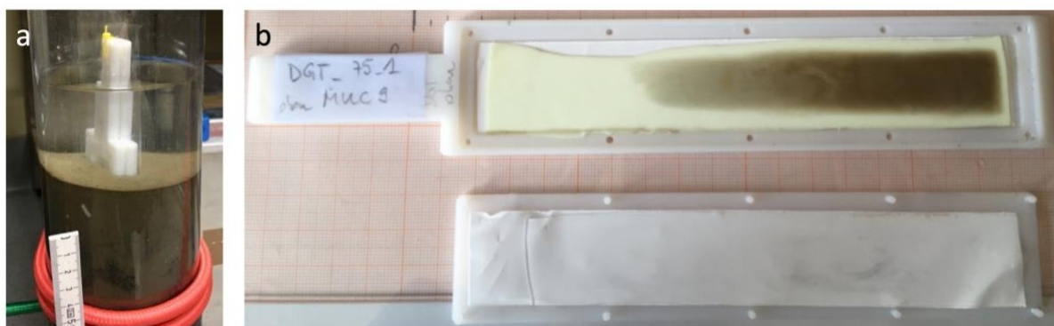
Fig. 5.2.4.2 (a) parallel back-to-back deployment of DET and DGT in one MUC core, (b) open DGT displaying the transparent diffusive gel at bottom picture half, and the sulfide-colored binding gel still in the sample holder, indicating a gradual and continuous increase of sulfide concentrations towards sediment depth, with absence of micro-niches.
