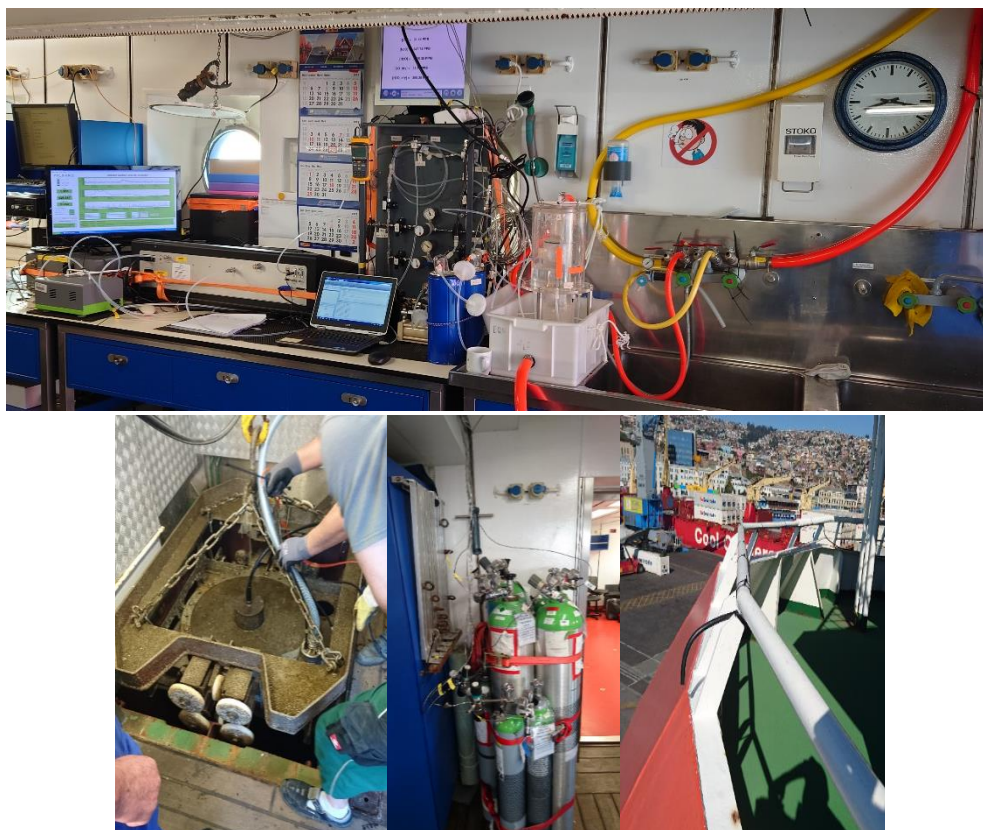
Fig. 5.11 Setup for underway measurements of trace gases during M189. (A) Equilibration system and gas analyzers, (B), reference gases, (C) submersible pump installed at the “moonpool” and (D) inlet for ambient air measurements.
