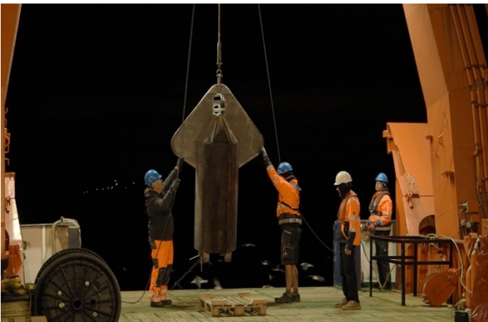
Fig. 12.4.3 Deployment of the head of CSEM streamer
