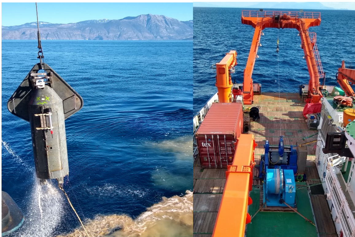
Fig. 5.1.4 Left: Depressor (pig) housing the transmitter electronics. Right: Werner Winch (dark blue winch towards the back of deck) with fiber-optical cable, that connects the transmitter electronics within the depressor to a control unit on the ship and also serves as a tow cable. The Toronto winch (light blue) is used to deploy and recover the receiver streamer.
