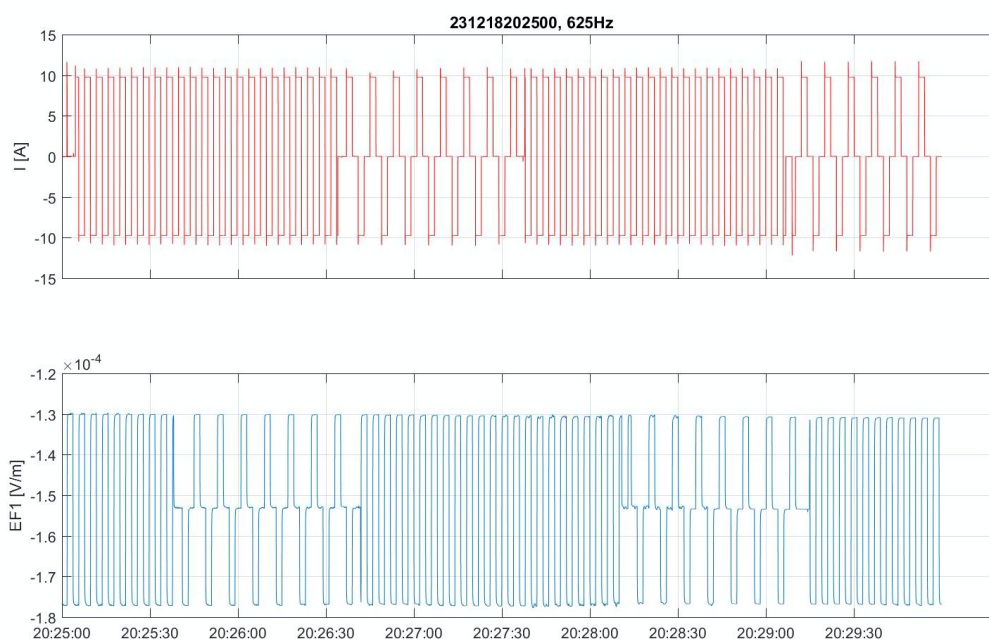
Fig. 5.1.10 5-minute time series example along Line 4. Top: transmitter signal, bottom: received signal at Receiver 1 (offset: 151.55m) while the seafloor array was not moving. Data quality is high for both, tow and stop sequences. The receiver data lost the synchronization with respect to the transmitter signal, which needs to be corrected in the post-processing.
