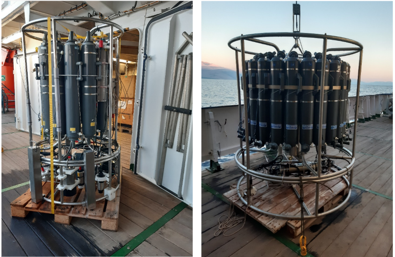
Fig. 5.2.1 GEOMAR Video-CTD/water sampler rosette device (left) and onboard CTD Device (right).
