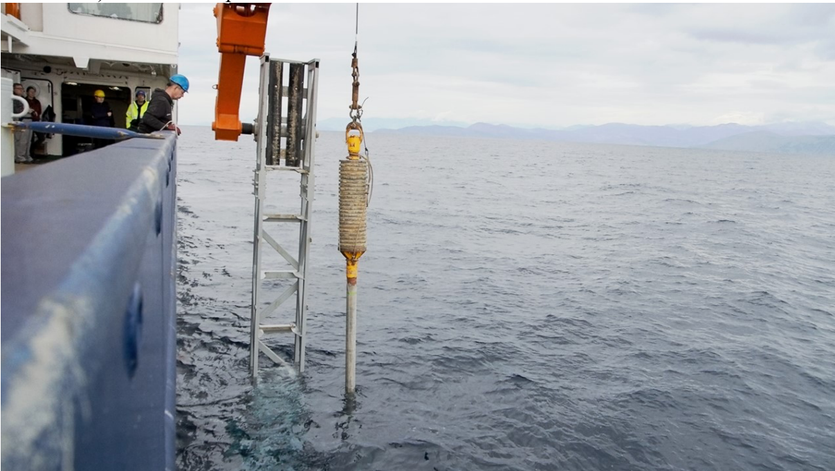
Fig. 5.3.1 Deployment of Gravity Core during M196 with the core handling rack of the METEOR.
