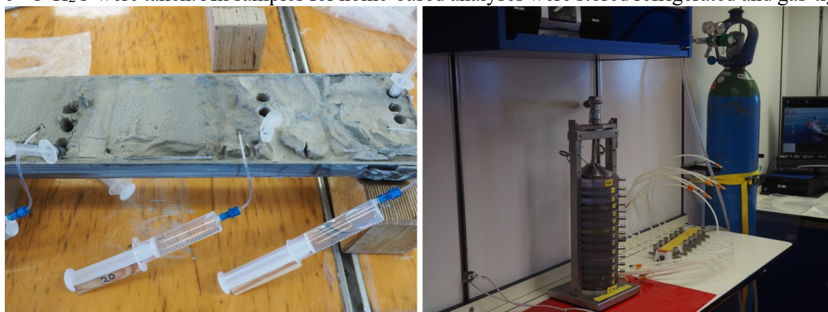
Fig. 5.3.5 Pore water sampling by Rhizon extraction (left) and with low-pressure squeezer(right).
