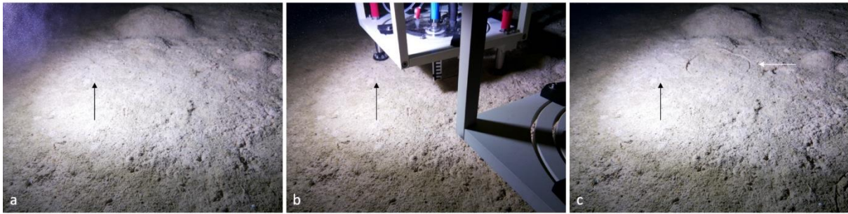
Fig. 5.8 Oblique view (camera 2) of (a) the sediment sampled by the left chamber of the DSR before the chamber is driven into the sediment, (b) during der flux measurement and (c) after the measurement when the chamber is retrieved out of the seafloor leaving a circular imprint in the sediment (white arrow). The black arrows indicate radial feeding tracks emanating from a small burrow entry hole.
