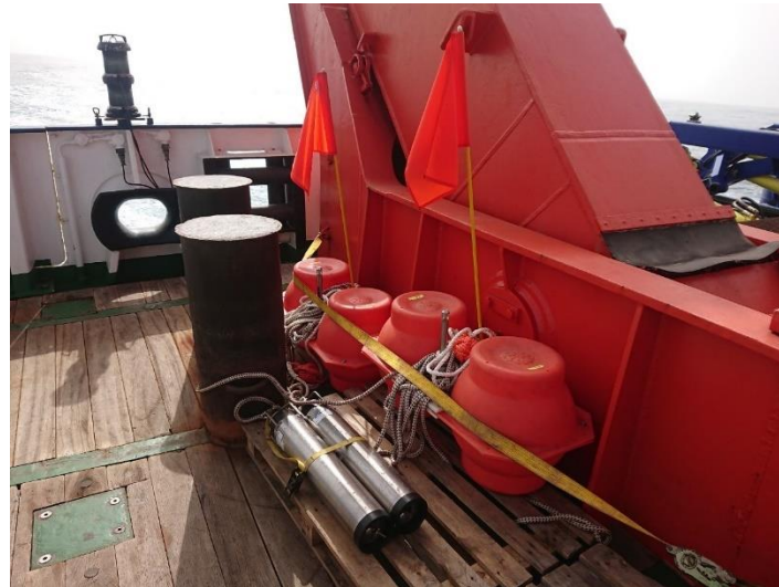
Fig. 12.6 LBL Transponders with floating spheres.
