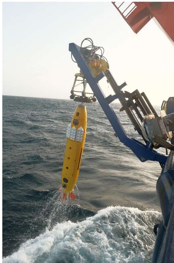
Fig. 12.3 Recovery of AUV Abyss with the LARS (launch and recovery system).
