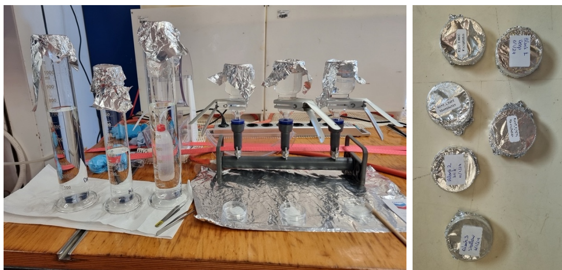
Fig. 5.02 Filtration system for water samples and petri dishes with dried filter papers ready for storage.
