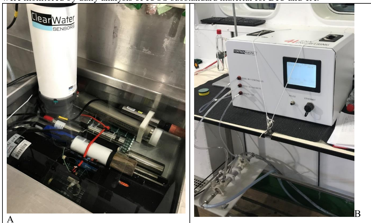
Figure 5.11. Sensors setup (A) and total alkalinity unit (B) connected to the underway system during MSM130 cruise.
