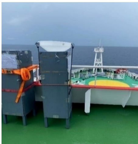
Fig. 5.9.2 The rainwater collector used on the cruise.
