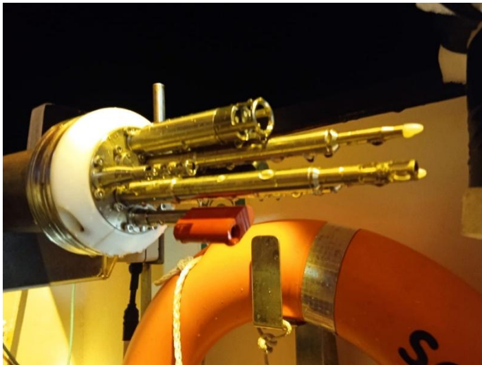
Fig. 4. Sensors at the tip of the microstructure profiler. Photo by Hannah Melzer.
