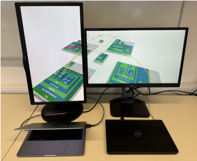
Fig. 3: Visualization of the distributed PetClinic on two monitors. The monitors are connected to different laptops running different operating systems.
