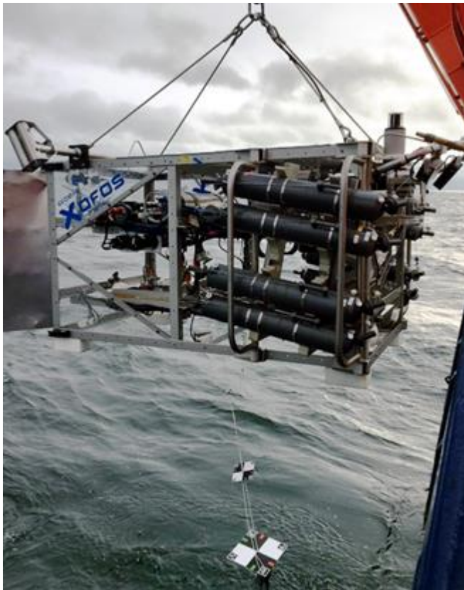
Fig. 5.18 Three color calibration boards are attached in the center of the XOFOS. They visualize light absorption and scattering.
