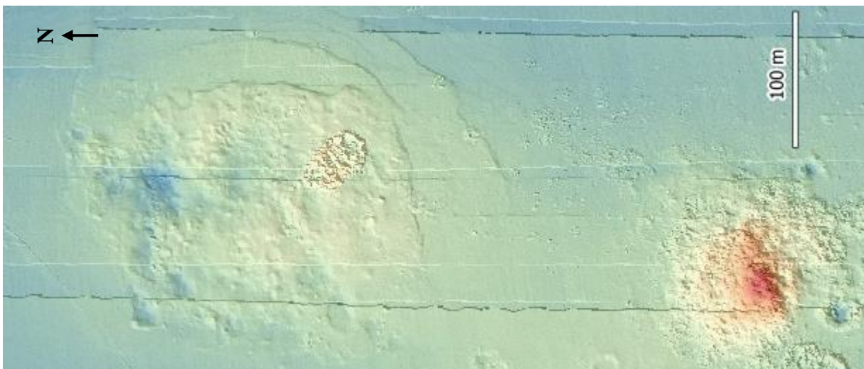
Fig. 5.13 Bathymetry data of the eastern part of the Pelzerhaken dumpsite. In this area, sediment is still dumped onto the seafloor.
