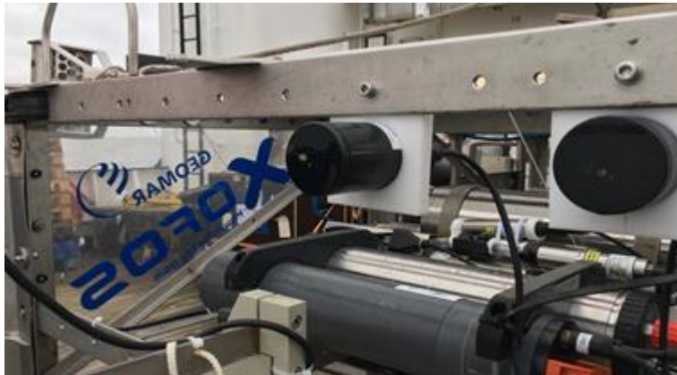
Fig. 5.17 ECO-VSFs mounted to XOFOS such that the sensors optical path is not obstructed by the frame.
