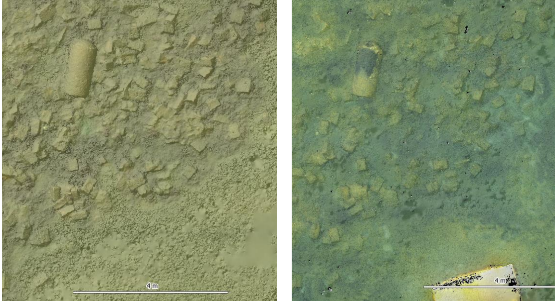
Fig. 5.4 Two photomosaics from the munition pile Pzh_00012 in Lübeck Bay. On the left side: A mosaic from July 2024 prior to clearance activities. On the right side: a mosaic in October 2024, after clearance activities.
