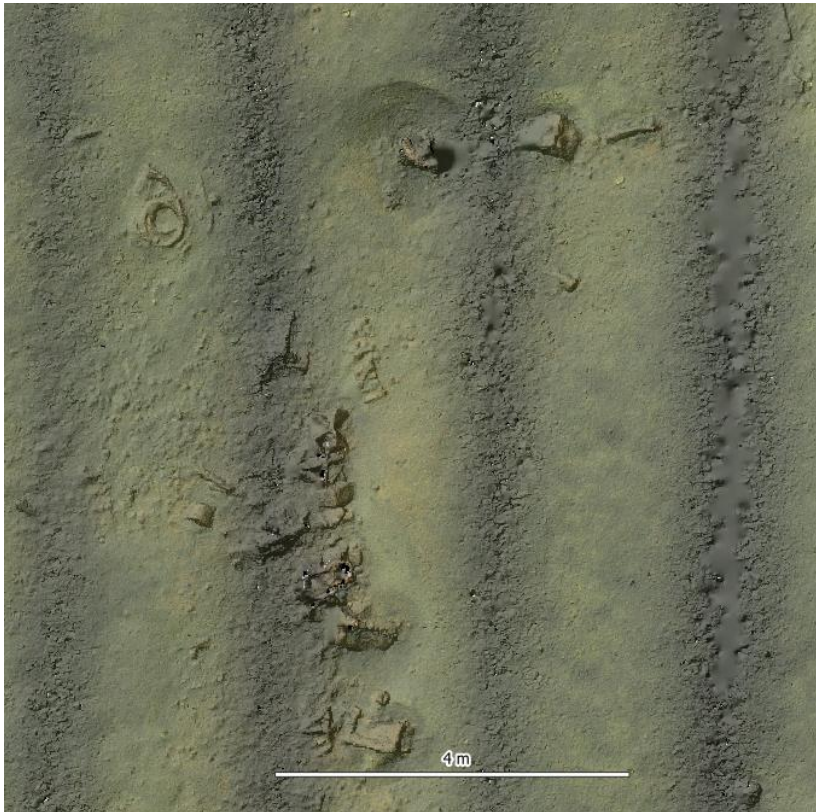
Fig. 5.5 Buried munition items in Lübeck Bay. To explain a large magnetic anomaly, even more munition has to be completely buried inside the sediment.
