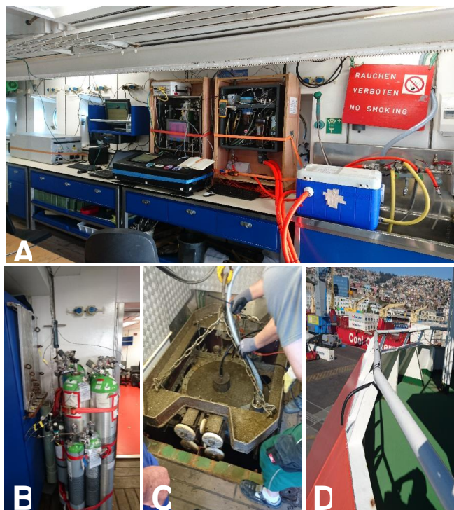
Fig. 5.5 Setup for UW measurements of \text{N}_2\text{O} concentration, \text{N}_2\text{O} isotopes, \text{CO}_2 , and \text{CO} during M148/1. (A) Equilibration system and gas analyzers, (B) inlet for ambient air measurements, (C) reference gases, (D) submersible pump installed at the “moon pool”.
