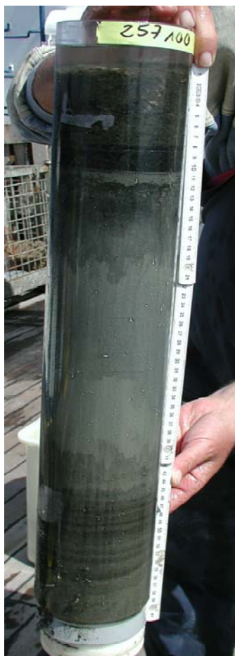
Figure 1 (IBSEN). Left: Core 257100 from the Gotland Basin (central Baltic Sea) taken in June 2003. This sediment core covers the last 1000 years in 60 cm. Three layers are visible: A black laminated layer on the bottom representing the MWP, a grey and homogeneous layer in the middle representing the LIA and a laminated black layer on top representing the present climate. Right: Vertical distribution of salinity and oxygen in the Gotland Sea as simulated with the model hierarchy for the three above periods.
