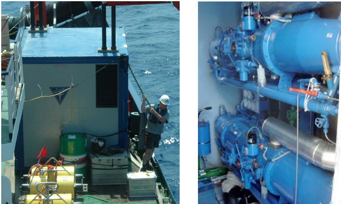
Fig. 6.2.1.1: Left: Junkers compressor container with Diesel tank Right: view inside the compressor container showing two of the four Junkers compressors.
