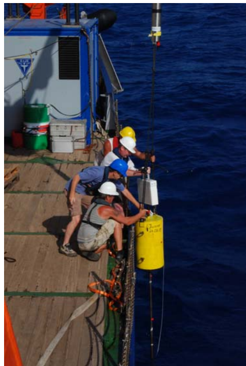
Fig. 6.5.1.3: After completion of assembly, the data acquisition box/ unit was attached to the hydraulic stab
