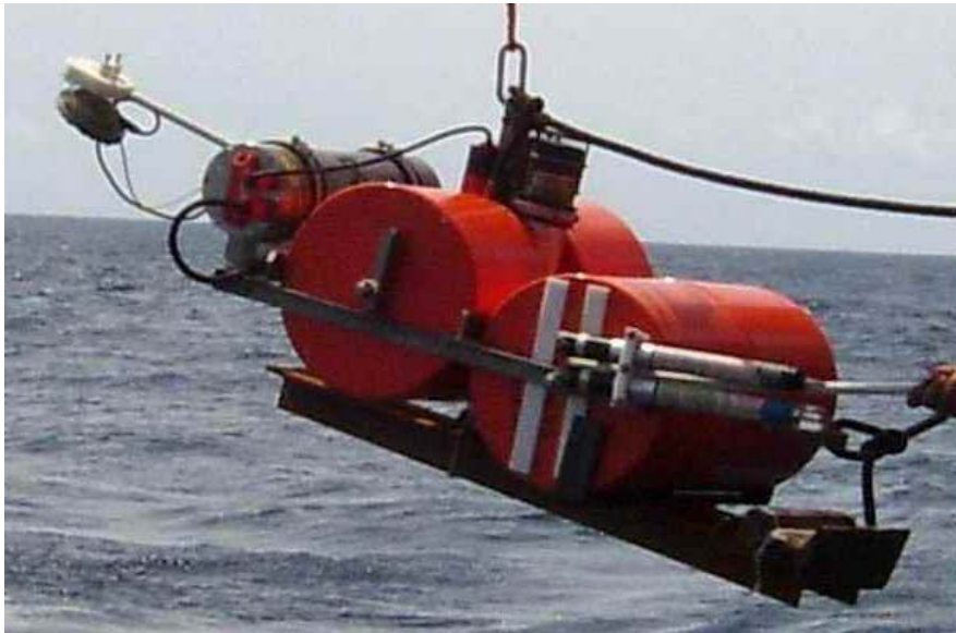
Figure 6.2.4.1: Ocean Bottom Seismometer – OBS - during deployment.
