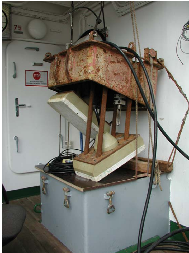
Figure 6.1.1: ELAC Bottomchart Mk. II 50-kHz transducers mounted in the moonpool of RV POSEIDON.
