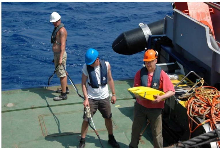
Figure 6.2.3.1.4: Floats are fixed on the cross cable in order to keep it at about 2 m depth during profiling
