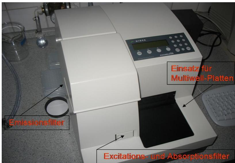
**Abb. 4 :** Plate Reader (Hidex, Plate Chameleon V, 425-106 Multilabel Counter)
