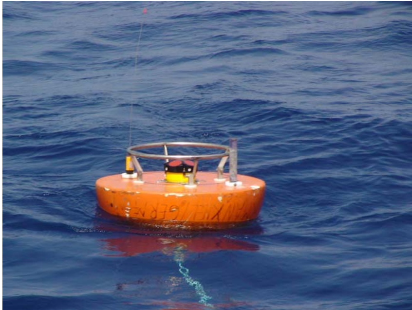
Fig. 4.7: Tip-Top element carrying the 1200 kHz ADCP atop the regular equatorial mooring at 23°W.
