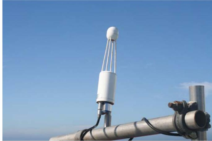
**Abb. 3.4:** LI-7500-Absorptionshygrometer (Licor).
